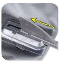
Slide skeg into the base. Skeg must go in far enough for locking clip slot to line up with skeg clip hole in skeg.
