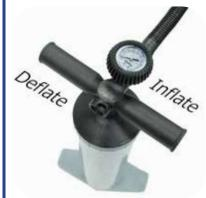
Some hand pumps have a lever to switch between single and double action mode. The Bravo 4 automatically bypasses double action mode when inflating beyond 6 PSI (Pounds per Square Inch).
