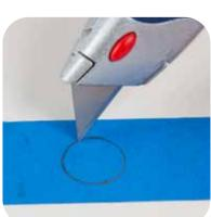
Pro Tip: Trace the outline of the penny on masking tape and cut with a utility knife. Apply tape to the boat instead of tracing on the boat.
